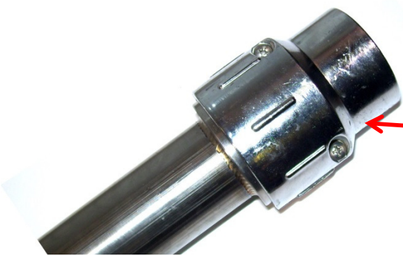
Gekko Tool Coupler Assembly Installed on Wand Tube (Apply Loctite 242 Medium Thread Locker to screws)
