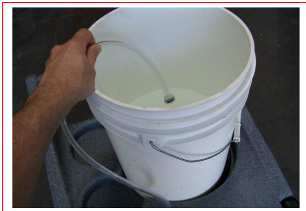
Place Chemical Feed Hose into Rinse Solution
