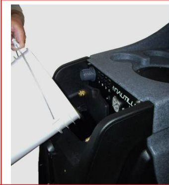
Pour appropriate amount of hot water into solution tank
