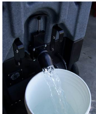
Drain Recovery Tank
