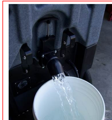
Drain water from Recovery Tank
