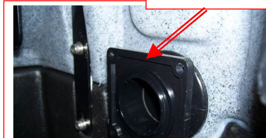
Unless damaged or leaking between tank and flange, the flange fitting does not have to be removed
