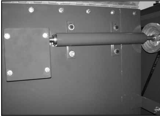
Worm drive shaft and pinion gear lubrication box
