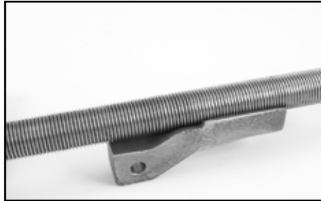
Fig. 2: Clutch block & feed screw
