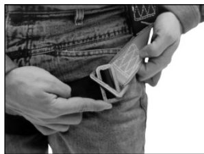
Figure 19A - Cross-over Style Harness Buckle Connections
