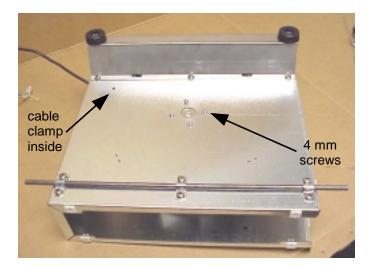
7. Remove the strain relief bushing holding the blower cable in the top of the base.
