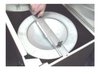
2. Push down on the filter hold-down bar and out on the back of the cabinet to disengage the two "ears" from the back of the cabinet. Rock the filter hold-down bar up towards the front of the cabinet.
