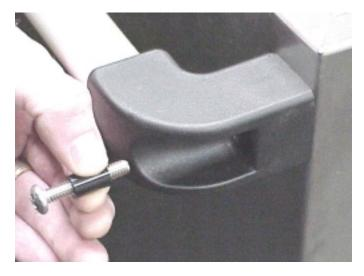
6. Place a ¼" lock nut into the hexagonal hole in the nut retainer and tighten with a Phillips screwdriver. Now tighten the small screw. Repeat this procedure on the other side.
