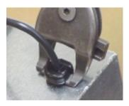
8. Using a pliers, twist the tabs of the base supports to align with the slots. Remove only one of the base supports (see below). Spread the base apart slightly to remove the blower.
