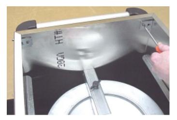
6. Slide one spacer over a ¼" x1¼" machine screw and insert them into the hole in the handle bracket.
