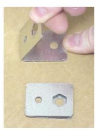
Place the nut retainers inside the back of the cabinet, as shown below. Using a Phillips screwdriver, thread a #10 x 5/8" screw through a nut retainer, the cabinet, and into the small boss on a handle bracket. Do not tighten completely.
