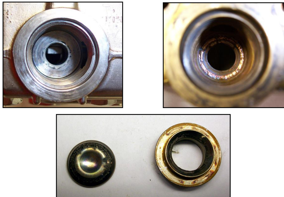
Figure 5-2. Inspect Manifold and Old Valves
