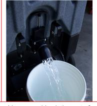
Vacuum acid solution out of Solution Tank
