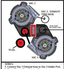
2. Place Plug in Base Exhaust Port. 3. Close Gate Valve.
