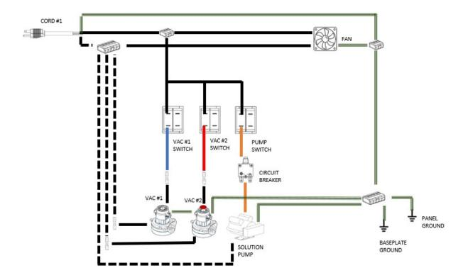
Nautilus MX-500M and MX3-500M wiring
