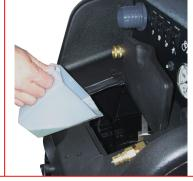
Add appropriate amount of chemical to water in solution tank
