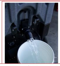
Drain water from Recovery Tank
