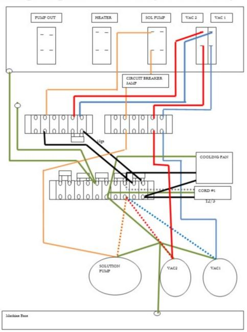
MX200 Wiring Diagram – Cord #1 (With Heater)
