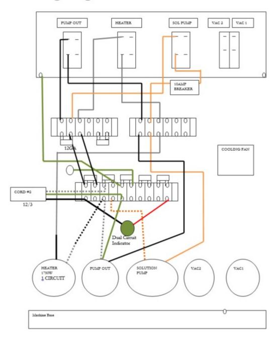
MX200 Wiring Diagram – Cord #1 (No Heater)
