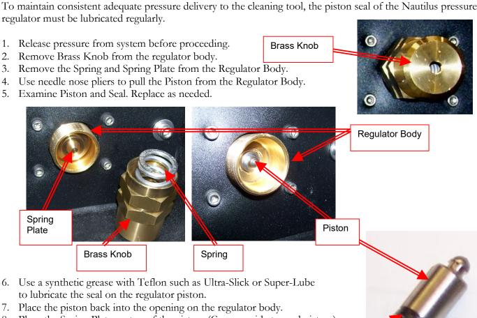
7. Place the piston back into the opening on the regulator body.
