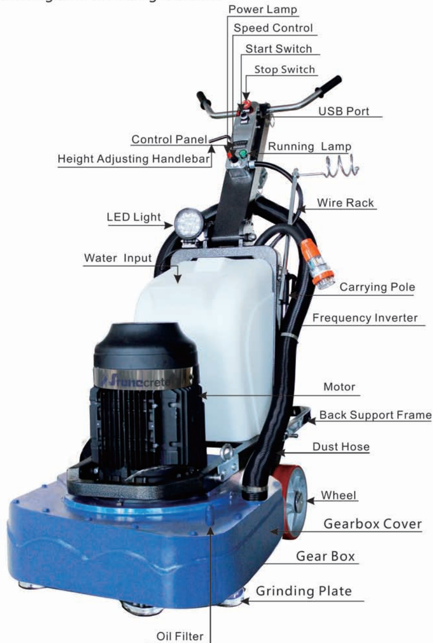
Q Series Diagram of Grinding Machine:
